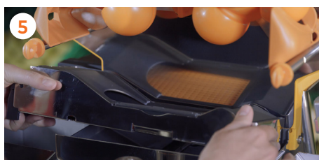
5 Take off the automatic PulpOut System , by lifting the assembly with the part closest to you.
