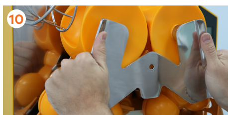
10 Remove the 1Step Extraction Kit by pulling it towards you with the stainless-steel handles.
