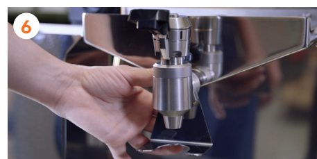
6 Remove the 2Services tap by easily unscrewing it.
