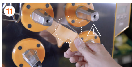
11 Remove the blade by pressing on the centre and pulling the handle towards you. Caution! Be careful not to cut yourself.
