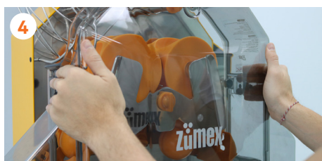
4 Turn the knobs and take off the front cover as well as the side outputs.
